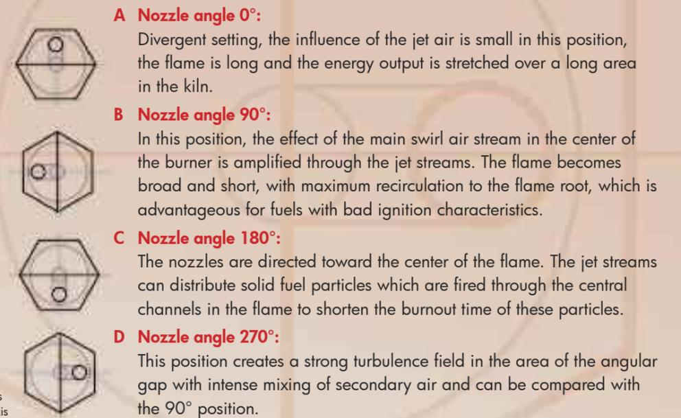
Fig. 2: various jet nozzle positions in relation to the burner axis
