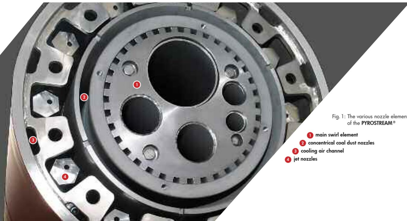
Fig. 1: The various nozzle elements of the **PYROSTREAM®**
