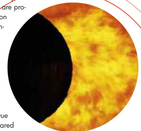
Fig. 3: Flame during heating of the kiln, jet nozzles turned into 90°-position resulting in a swirl in clockwise direction
