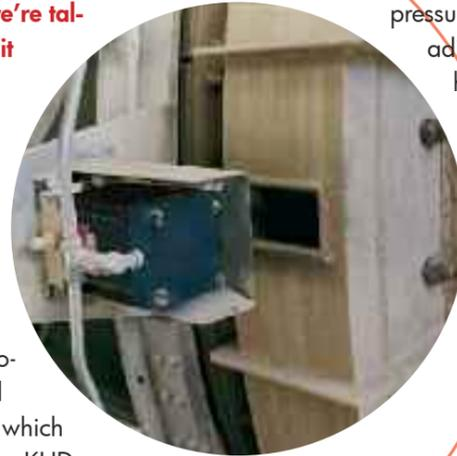
The kiln inlet area with pneumatically-operated seal...
