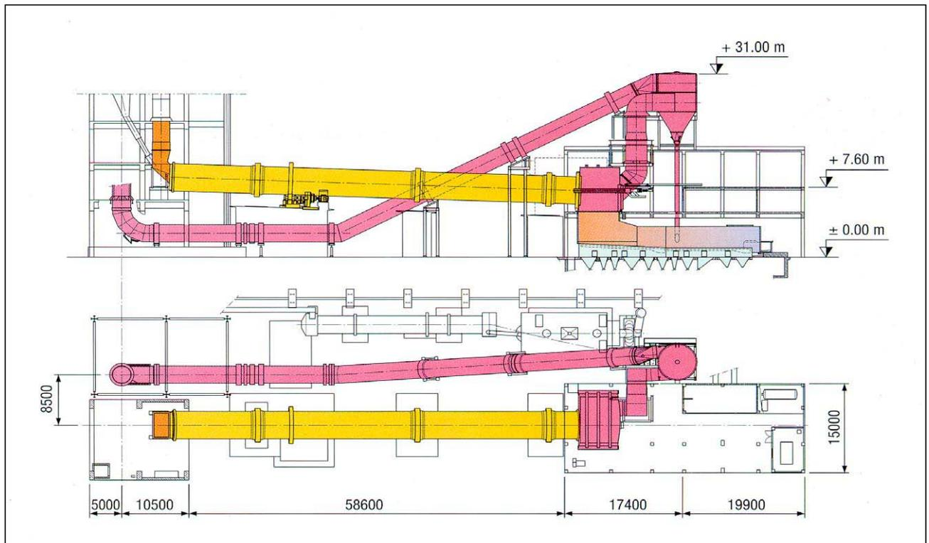
Figure 4: Existing rotary kiln with new installed tertiary air duct, dust chamber, extended kiln hood and grate cooler.
