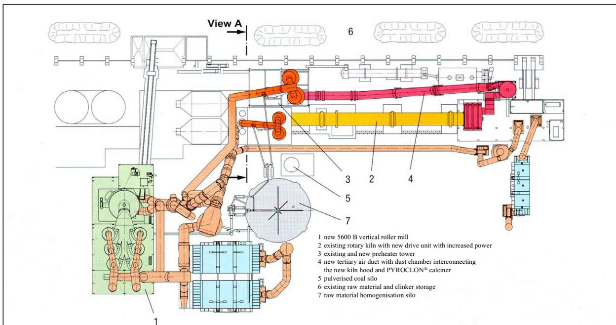
Figure 1: General layout of production line no. 4 at Adana.
