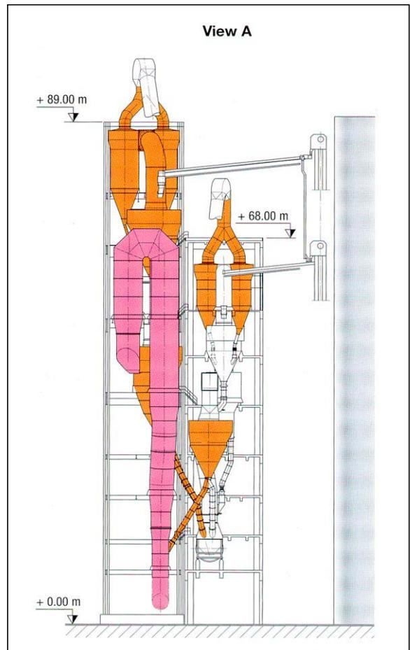
Figure 3: Layout of the existing preheater system and newly installed preheater with PYROCLON®-calciner.
