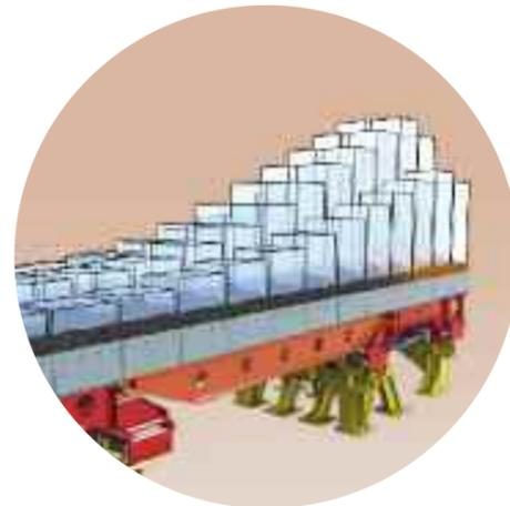
Aeration of the **PYROFLOOR**<sup>®</sup> cooler is locally optimized
