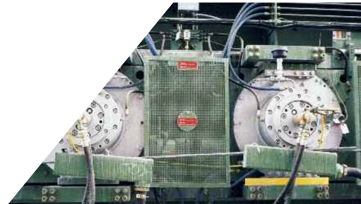
Bearing housing and guide for the movable and fixed roll, bearing lubrication using oil circulation
