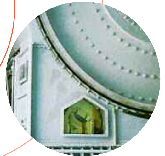
Mill with slide shoe bearings and inspection window
