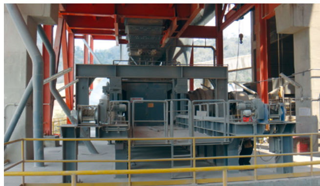
A RP-M 18-200/180 roller press is the core of the raw grinding system
