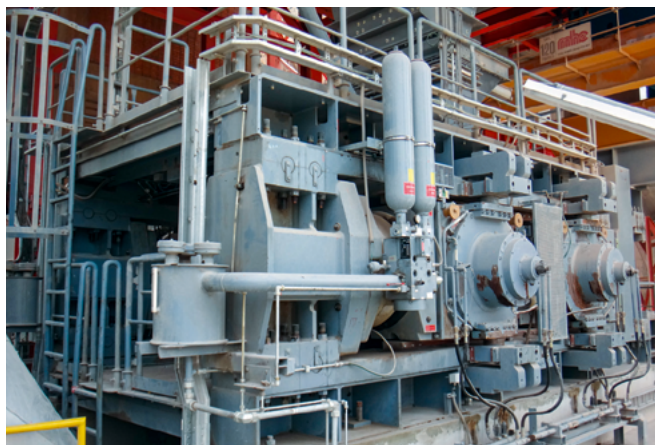
A RP-M 18-200/180 roller press is the core of the raw grinding system
