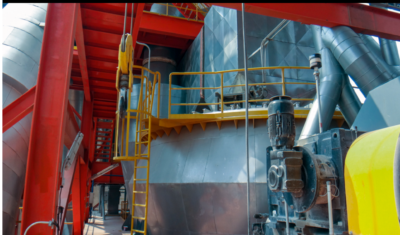
KHD supplied VS 620 and LS 8600 separators for coarse and fine particle separation, respectively
