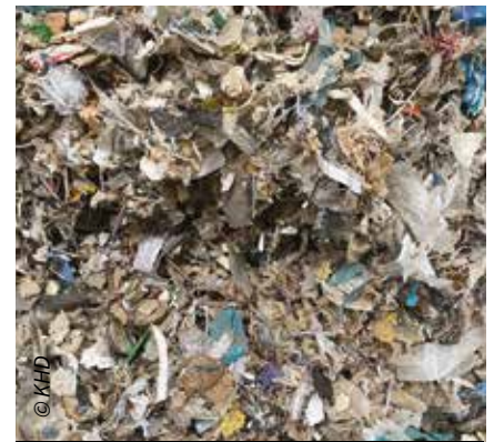
Figure 3: coarse waste-derived fuel (WDF) can be fed into the Pyrorotor without pre-processing thanks to high residency time that allows for complete burn-out
