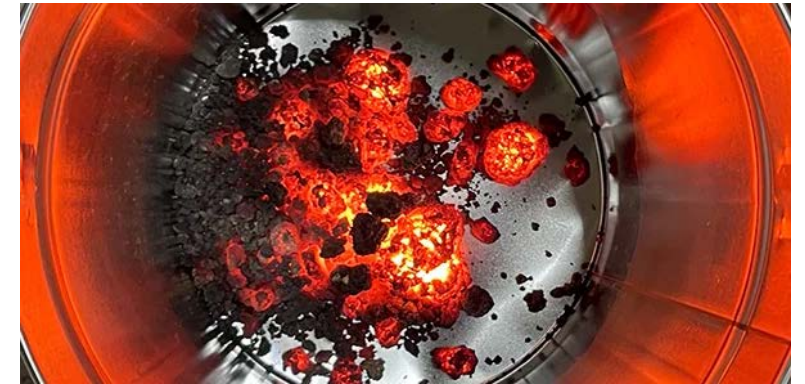
Electric plasma-burner in experimental kiln of consortium partner Heidelberg Materials
